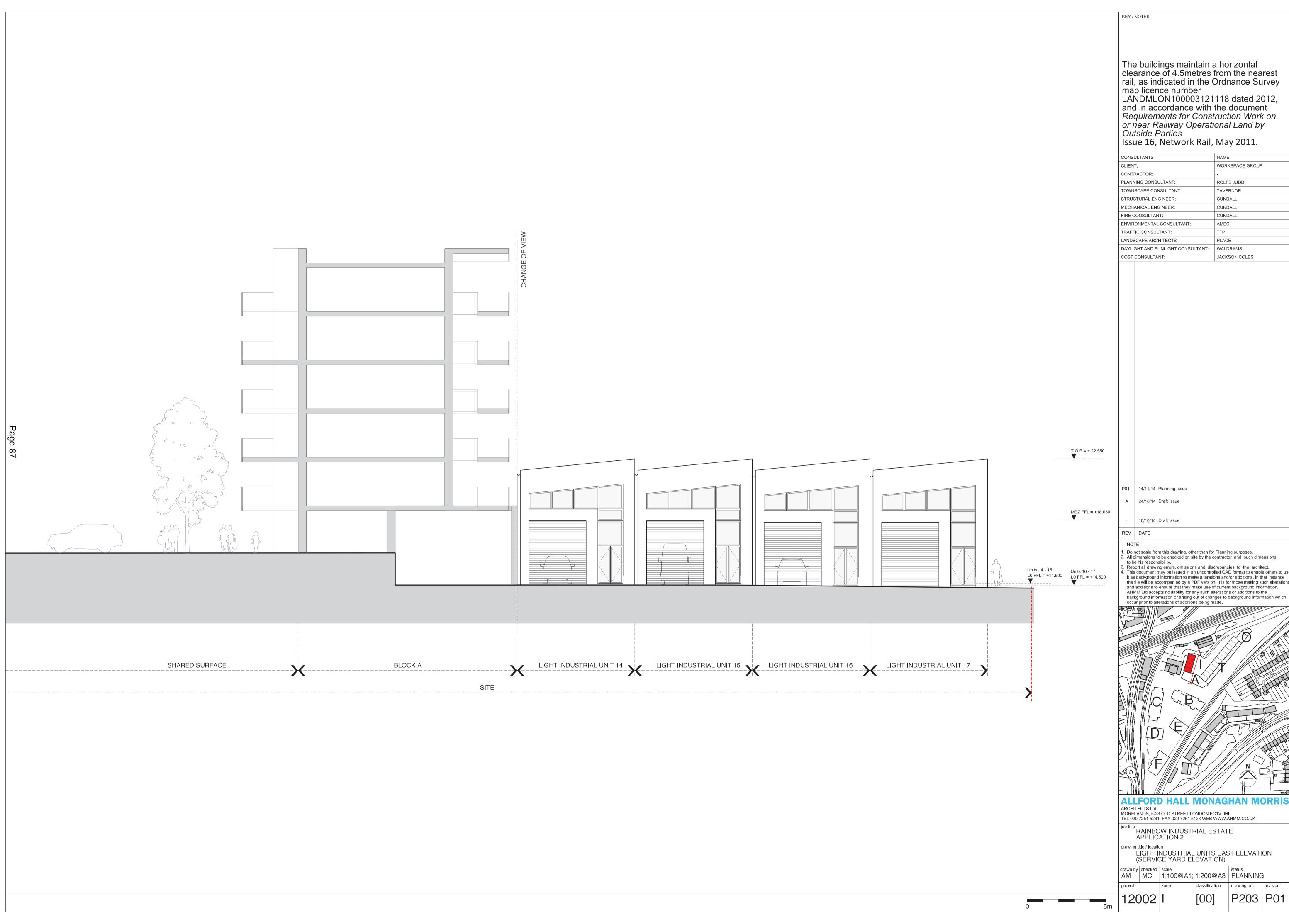
The buildings maintain a horizontal clearance of 4.5metres from the nearest rail, as indicated in the Ordnance Survey map licence number LANDMLON100003121118 dated 2012, and in accordance with the document Requirements for Construction Work on or near Railway Operational Land by Outside Parties Issue 16, Network Rail, May 2011.
